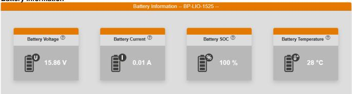
Battery Voltage: Shows the actual battery voltage of the battery or energy storage.
