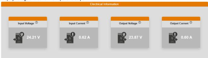
Input Voltage: Shows the actual input voltage of the UPS. Input current: Shows the actual input current of the UPS. Output voltage: Shows the actual output voltage of the UPS. Output current: Shows the actual output current of the UPS.
