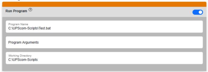
When enabled, it can run a batch or a program after shutdown by time or SOC.
